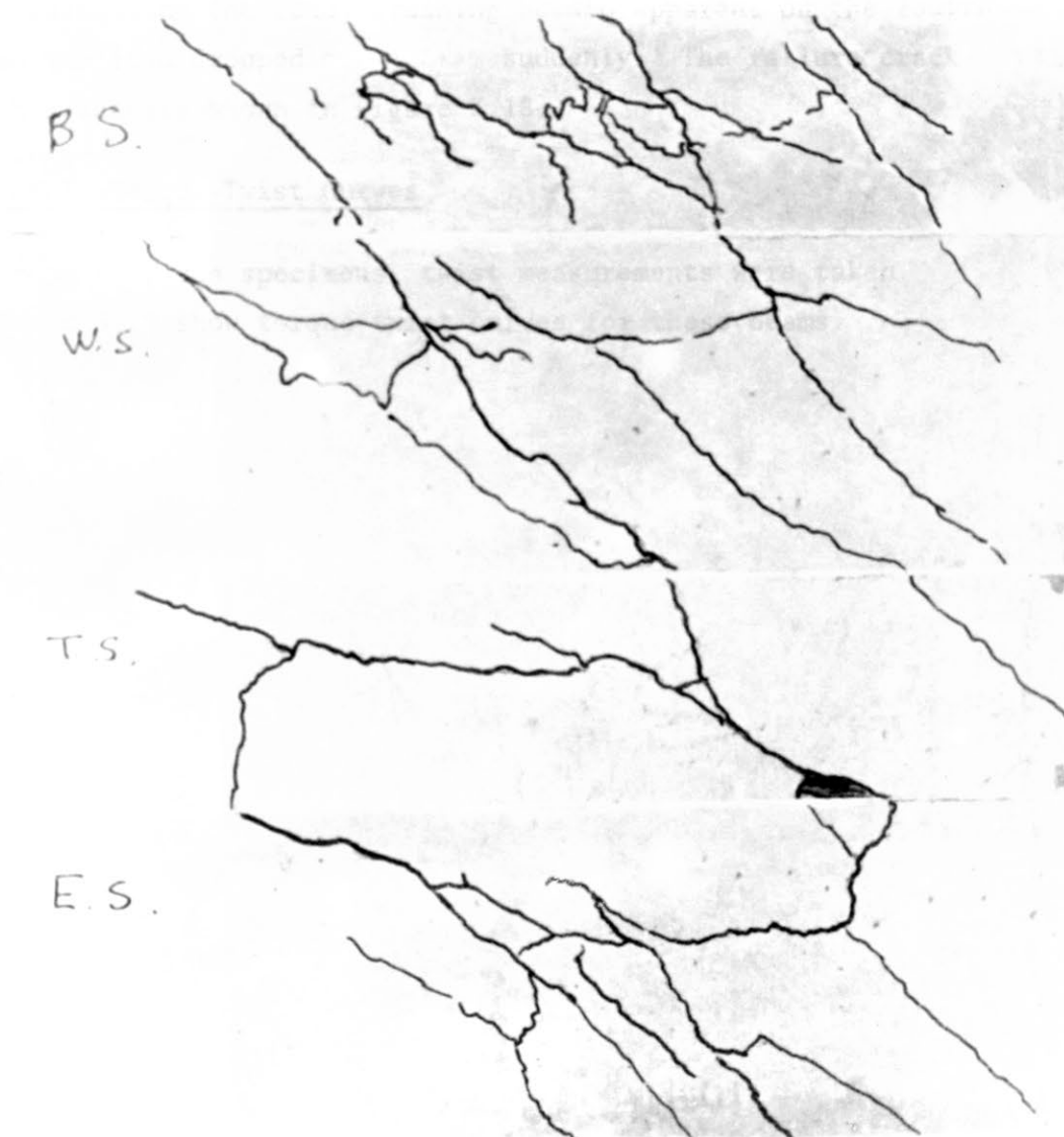
FIG.3.17 DEVELOPED FAILURE SURFACE OF BEAM 36T4c MODE 3 FAILURE
