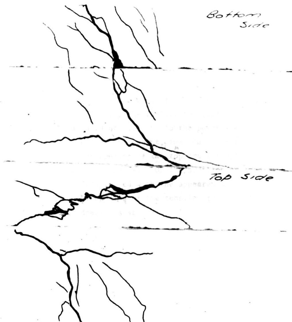
FIG. 3.16 DEVELOPED FAILURE SURFACE BEAM 36T4 MODE 1 FAILURE.
