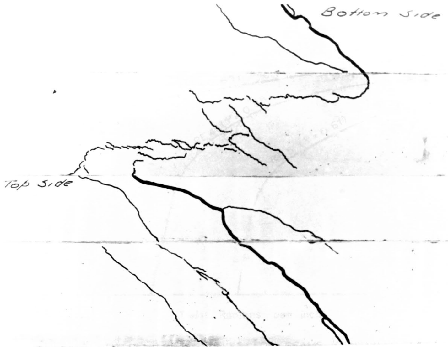
FIG.3.18. DEVELOPED FAILURE SURFACE OF BEAM 38T5 MODE 2 SURFACE.
