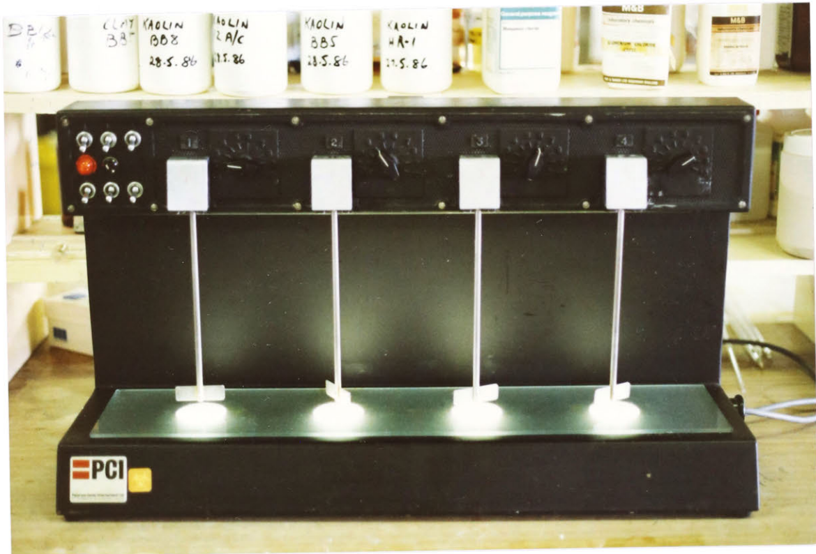
Figure 3.1 The jar test apparatus used in the study
