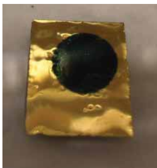
Figure 6.7: A picture of the 0,05C PEDOT/pTS film deposited on the gold substrate bearing PHEMA brushes.
